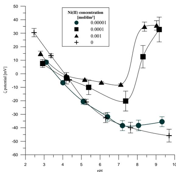
Fig. 6.  $\zeta$  potential at Fe<sub>2</sub>TiO<sub>5</sub> / NaCl solution interface as a function pH
