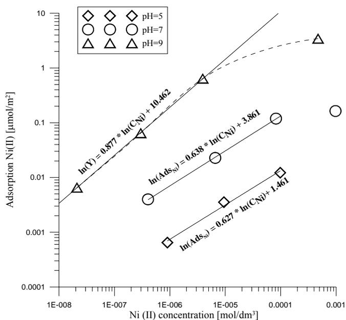
Fig. 4. Adsorption of Ni (II) at Fe<sub>2</sub>TiO<sub>5</sub>/0.001 NaCl solution interface as a function of equilibrium concentration for selected pH values (5, 7 and 9)
