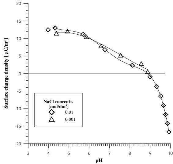
Fig. 1. Surface charge density at the Fe<sub>2</sub>TiO<sub>5</sub>/NaCl solution interface as a function of pH
