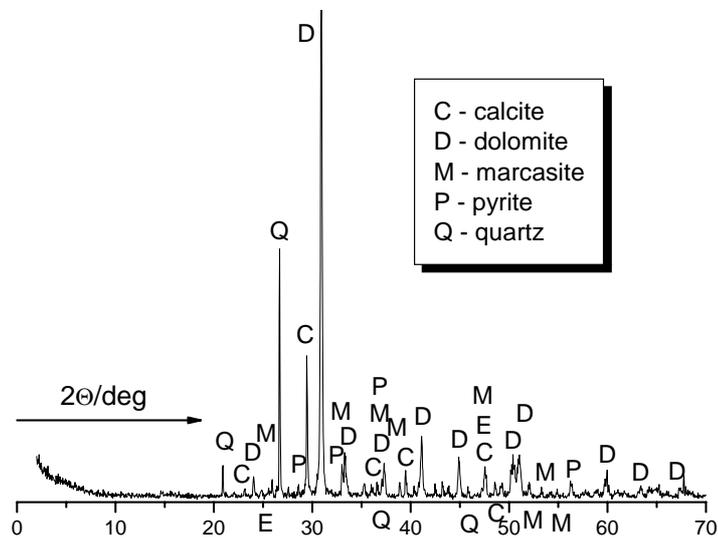
Fig. 1. X-ray diffraction pattern of investigated flotation tailings
