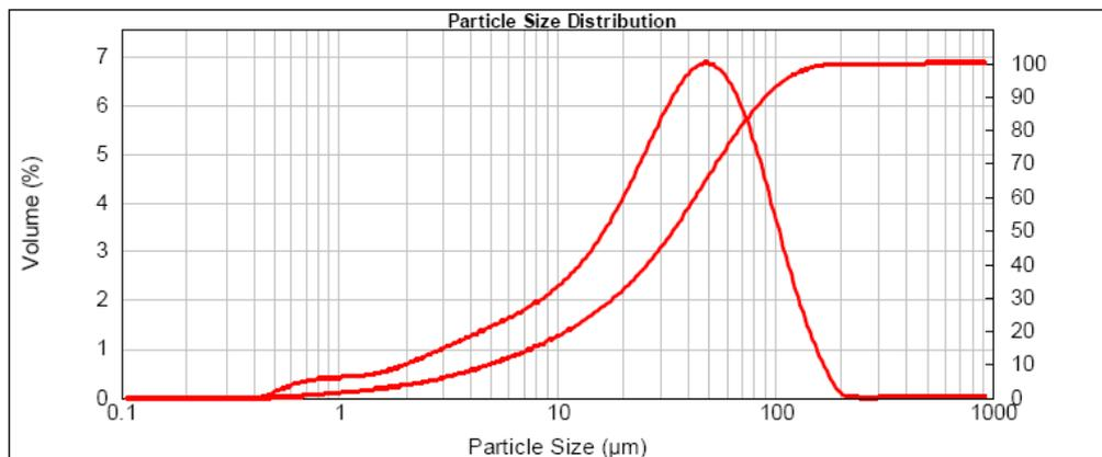
Fig. 1. Particle size distribution of black shale sample "A"
