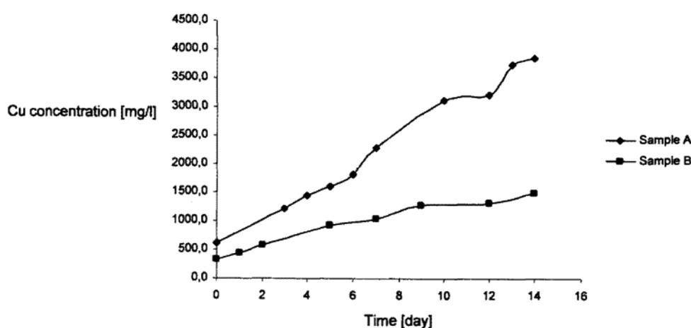
Fig. 4. Autotrophic bioleaching of black shale samples
