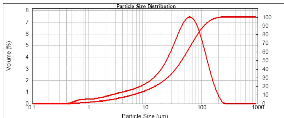
Fig. 2 Particle size distribution of black shale sample "B"
