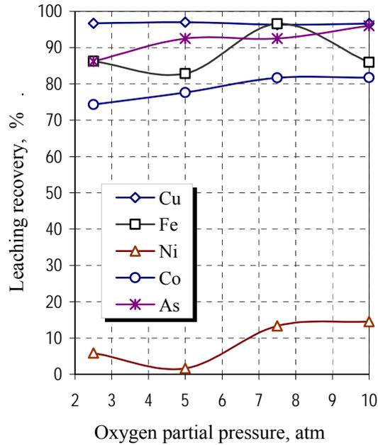
Fig. 7. Effect of oxygen partial pressure on metals recovery from Lubin middlings. Temperature 140 °C, H<sub>2</sub>SO<sub>4</sub> 50 g/l, s/l 1:10 (1 atm = 0.101 MPa)
