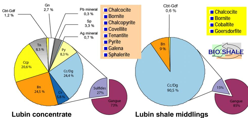
Fig. 1 . Mineralogical composition of Lubin copper sulphide concentrate and shale middlings tailings of 1<sup>st</sup> cleaning flotation (BRGM data, Auge et al., 2007)
