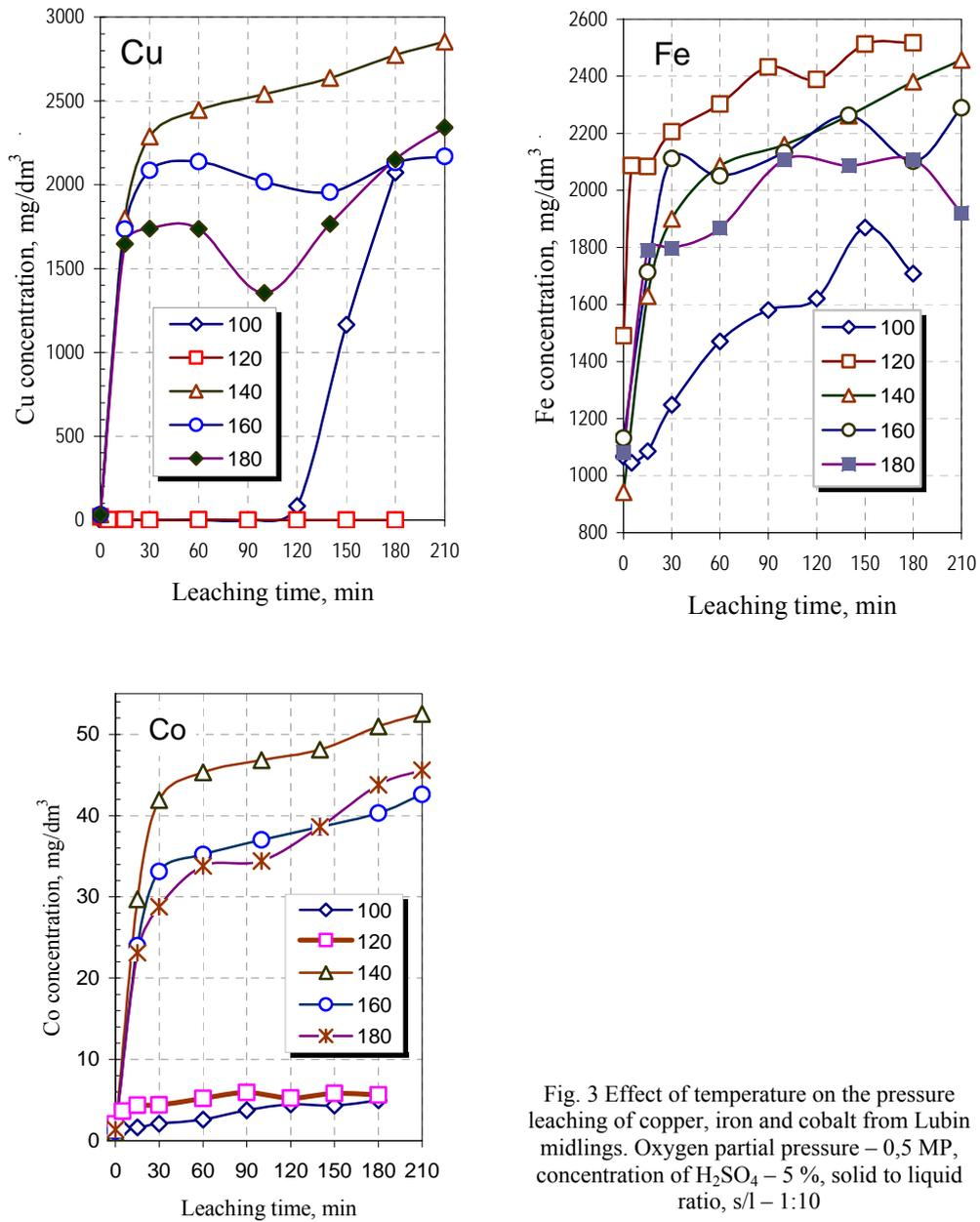
Fig. 3 Effect of temperature on the pressure leaching of copper, iron and cobalt from Lubin midlings. Oxygen partial pressure – 0,5 MP, concentration of H<sub>2</sub>SO<sub>4</sub> – 5 %, solid to liquid ratio, s/l – 1:10
