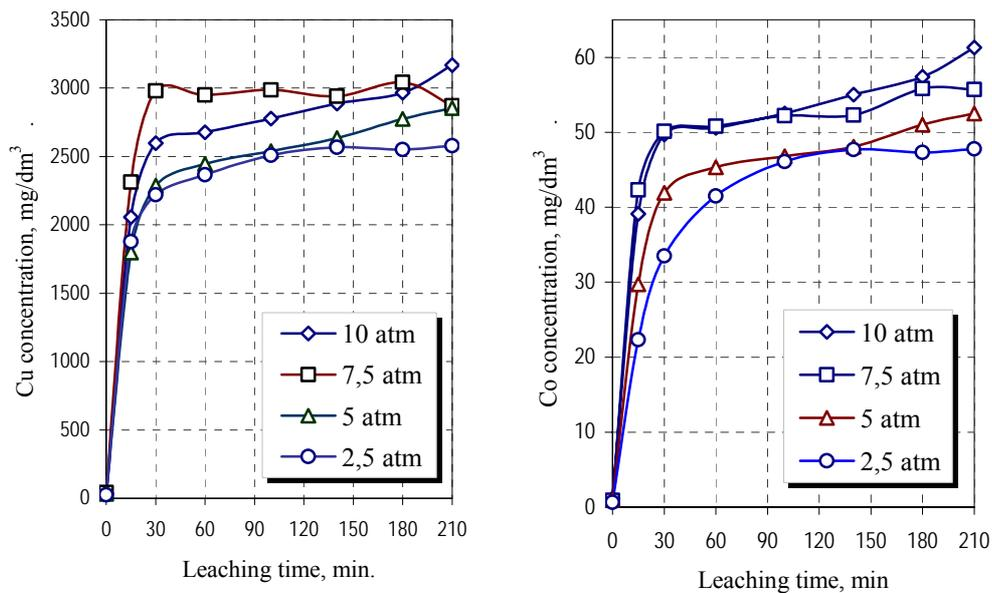
Fig. 6. Effect of oxygen partial pressure on Cu and Co leaching rate for the pressure leaching of Lubin middlings. Temperature 140 °C, Concentration of H<sub>2</sub>SO<sub>4</sub> 5 %, Liquid/solid ratio 10:1
