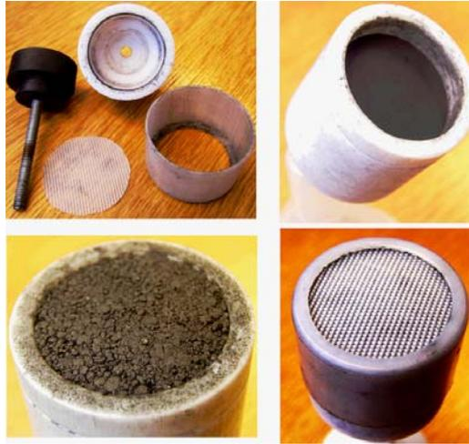
Fig. 4. Construction of the graphite paste electrode
