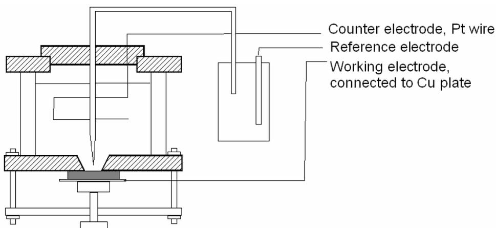
Fig. 1. Simplified diagram of the Avesta cell
