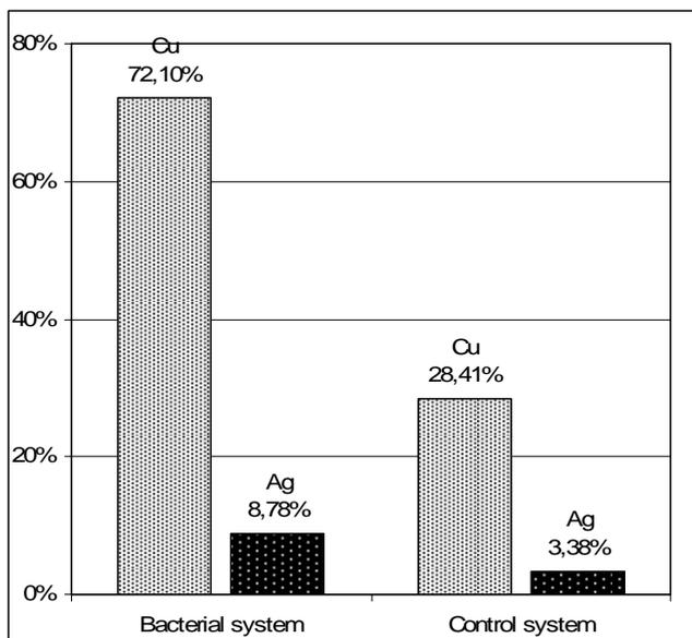
Fig. 3. Percentage of Cu and Ag extracted from pretreated ore (25 days heterotrophic treatment) after 35 days autotrophic bioleaching (process 2 – stage 2: autotrophic bioleaching)
