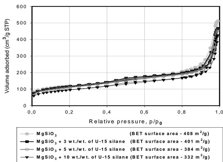
Fig.5. N<sub>2</sub> adsorption/desorption isotherms of the examined magnesium silicates precipitated from MgSO<sub>4</sub> solution modified with aminosilane U-15
