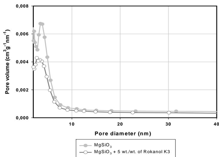
Fig. 2. Pore size distribution (BJH method) of the examined magnesium silicates precipitated from  $MgCl_2$  solution
