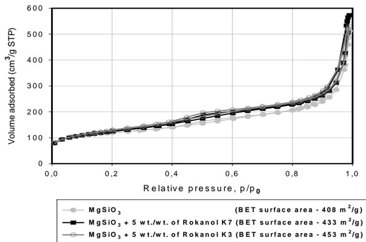
Fig. 4. N<sub>2</sub> adsorption/desorption isotherms of the examined magnesium silicates precipitated from MgSO<sub>4</sub> solution
