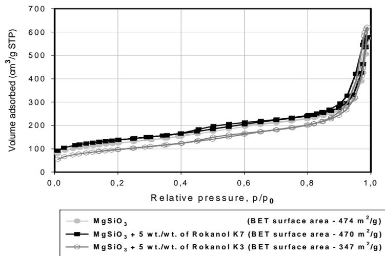
Fig. 3. N<sub>2</sub> adsorption/desorption isotherms of the examined magnesium silicates precipitated from Mg(NO<sub>3</sub>)<sub>2</sub> solution
