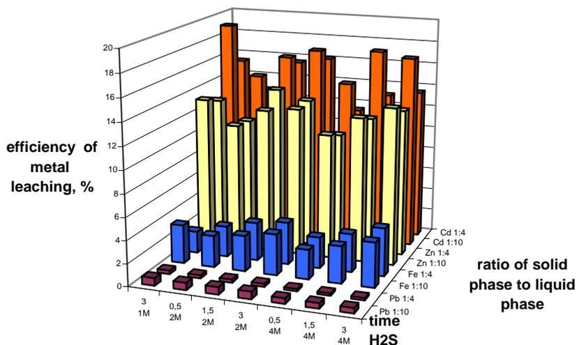
Fig. 2. Influence of time, H<sub>2</sub>SO<sub>4</sub> concentration, solid phase to liquid phase on the efficiency of leaching of Cd, Fe, Pb and Zn from Zn-Pb flotation tailings
