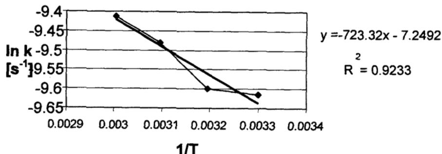
Fig. 5. Arrhenius diagram for determining activation energy
