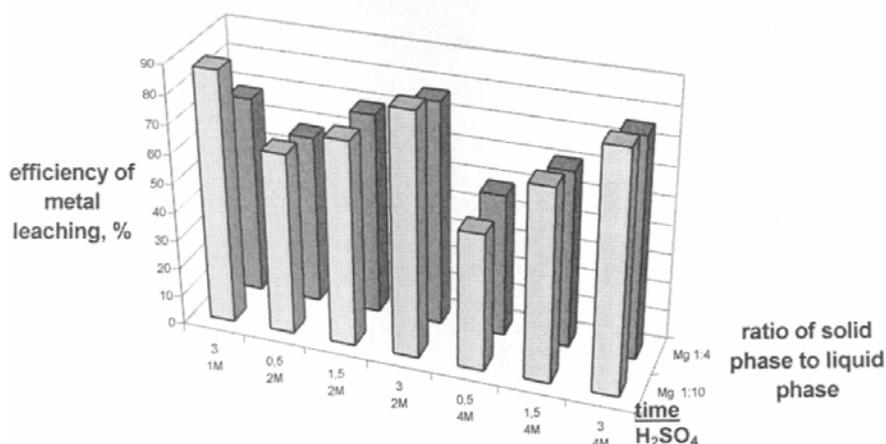
Fig. 1. Influence of time, H<sub>2</sub>SO<sub>4</sub> concentration, solid phase to liquid phase on the efficiency of magnesium leaching from Zn-Pb flotation tailings
