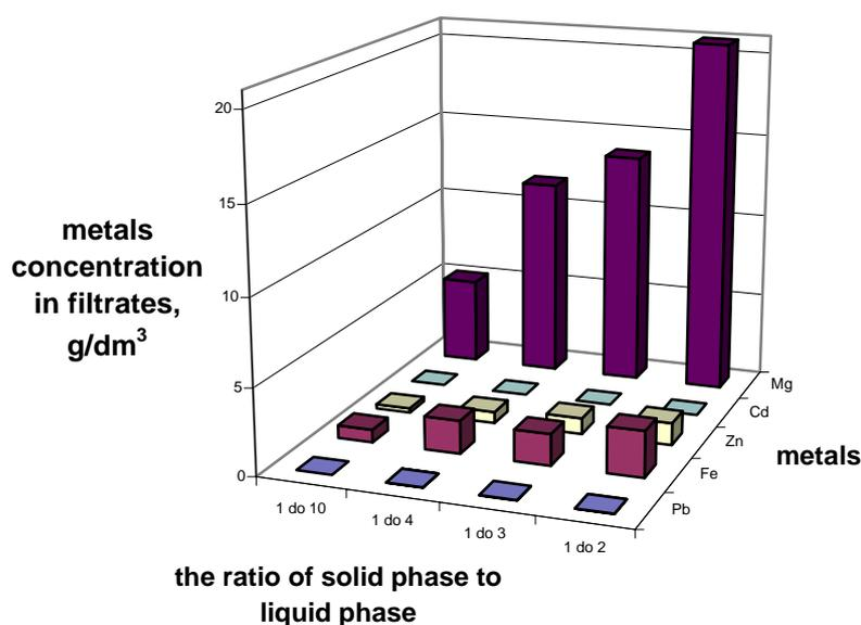
Fig. 3. Metal concentration in the solution at different solid/liquid phases ratios, the temperature of 293 K, 2 M H<sub>2</sub>SO<sub>4</sub>, 3 hours
