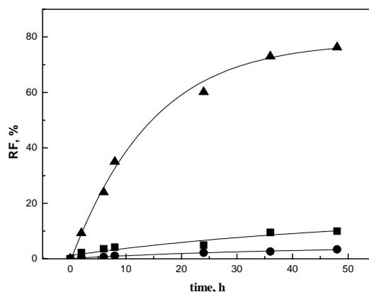
Fig. 3. Recovery of Zn(II), Cd(II), and Pb(II) ions from source phase from aqueous solutions in transport across PIM with azocrown ethers **3**. Source phase:  $c_{\text{Me(II)}} = 0.001$  M each; pH = 5.0; receiving phase: 1.0 M HCl; membrane:  $2.60 \text{ cm}^3$  *o*-NPPE / 1 g CTA, 0.05 M of azocrown (based on plasticizer volume)
