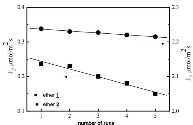
Fig. 5. Initial flux vs. number of run in repeated transport of Pb(II) ions across PIM with carriers 1 or 2; source phase:  $[\text{Pb(II)}]=[\text{Cd(II)}]=[\text{Zn(II)}]=0.001\text{M}$  each, receiving phase: 1.0 M HCl; membrane:  $2.60\text{ cm}^3$  *o*-NPPE / 1 g CTA, 0.05 M of azocrown (based on plasticizer volume)
