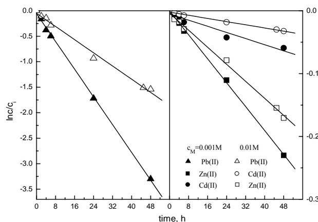
Fig. 4. Relationship of  $\ln c/c_i$  vs. time for Pb(II), Cd(II) and Zn(II) transport across PIMs with **2** from source phase of different metal ions concentration; receiving phase: 1.0 M HCl; membrane:  $2.60 \text{ cm}^3$  *o*-NPPE / 1 g CTA, 0.05 M of azocrown (based on plasticizer volume)
