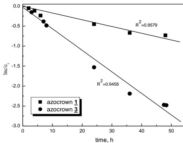
Fig. 2. Kinetics of Pb(II) ions transport across PIMs containing 0.05 M of azocrown ethers **1** or **3** from aqueous solutions. Source phase:  $c_{\text{Pb(II)}} = 0.001$  M; pH = 5.0; receiving phase: 1.0 M HCl; membrane: 2.60 cm<sup>3</sup> *o*-NPPE / 1 g CTA, 0.05 M of azocrown (based on plasticizer volume)
