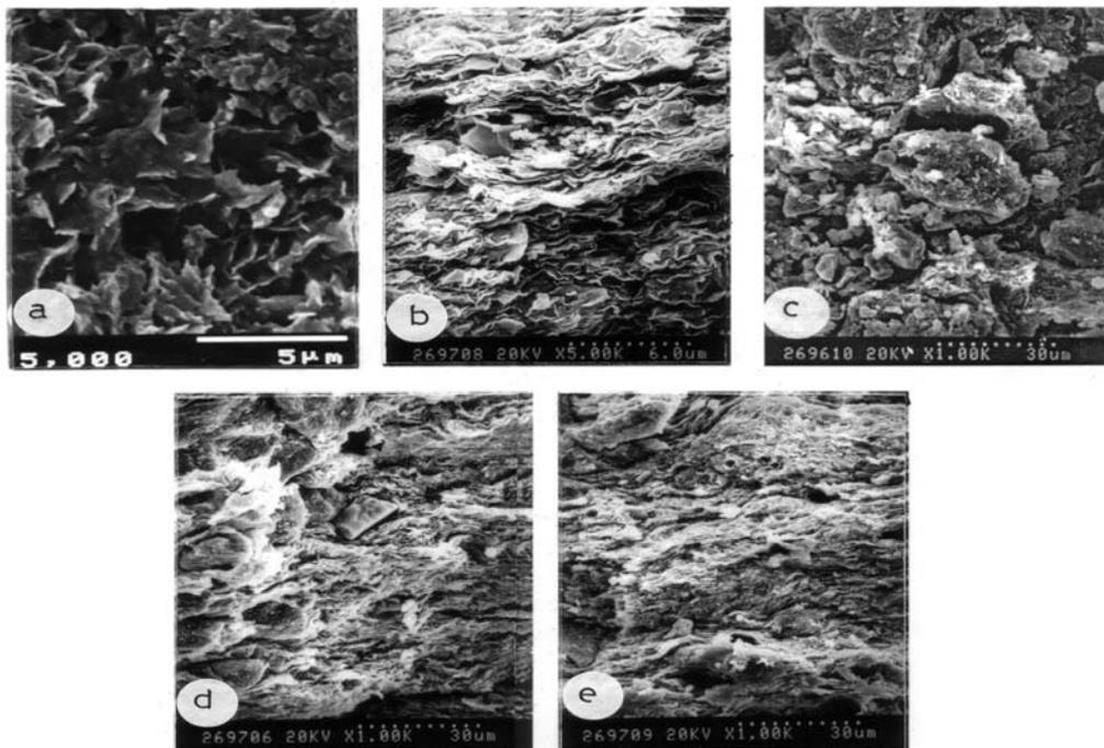
Fig. 3. Scanning Electron Microscope microphotographs of representative clayey sediments
