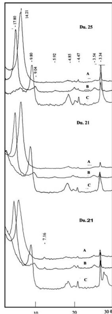
Fig. 2. Diffractogram of the representative clay fraction of the Upper Cretaceous sediments of Abu Tartur Plateau
