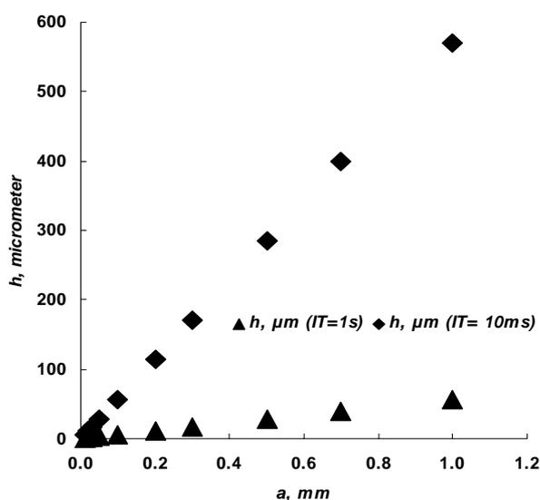
Fig. 3. Diameter of the rupturing film dependence of the critical thickness of the rupturing wetting film
