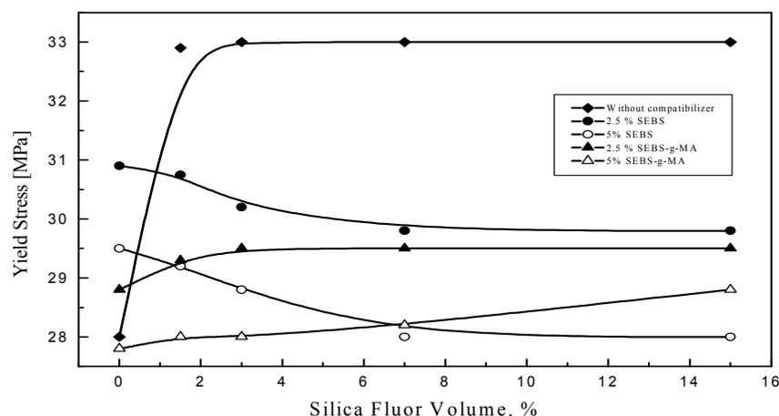
Fig. 6. Influence of silica content on the yield stress of filled-PP blends
