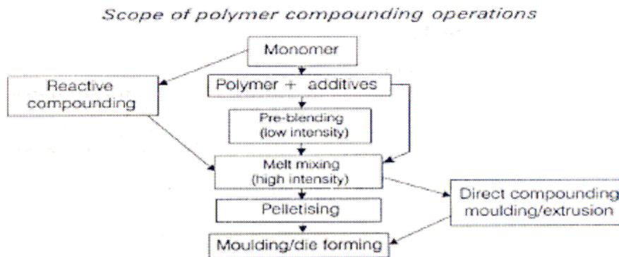
Fig. 2. Scope of Various Compounding Operations (O'Driscoll, M., 1994)
