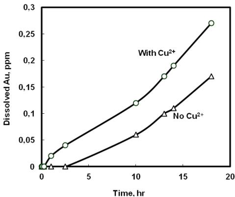
Fig. 9. Dissolution of pure gold wires (0.1 g) in presence and absence of  $\text{CuSO}_4$  at different time periods. Leaching solution:  $200 \text{ cm}^3$  containing 0.1 mM  $\text{CuSO}_4$ , 0.3 M AH, 0.2 M ATS. Shaking speed: 480 rpm at ambient temperature and sealed vessel
