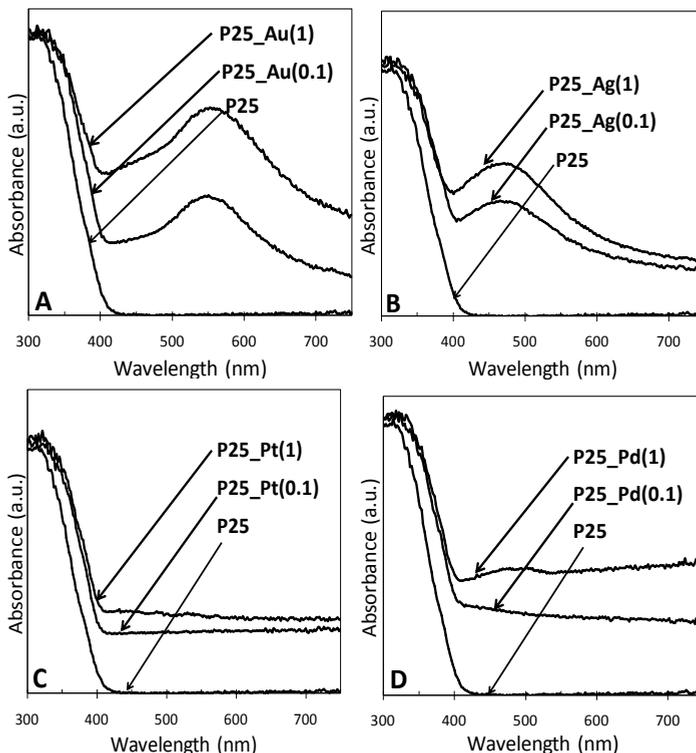
Fig. 3. Diffuse reflectance spectra of pure and: (A) gold- (B) silver (C) platinum (D) palladium-modified TiO<sub>2</sub>
