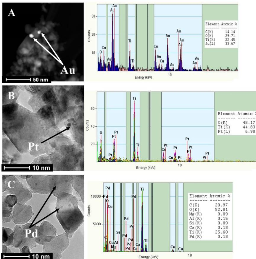
Fig. 2. EDS mappings of 1 % (m/m) (A) gold- (B) platinum (C) palladium-modified TiO<sub>2</sub>
