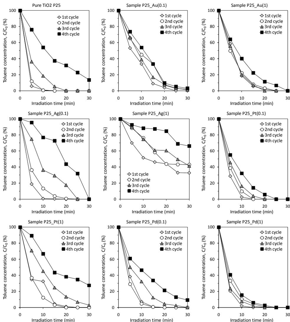
Fig. 4. Toluene photodegradation efficiency as the function of irradiation time. The influence of kind and amount of metal precursor on the initial photocatalytic activity of TiO<sub>2</sub> nanotubes and their stability in four measurement cycles under UV-Vis LEDs irradiation
