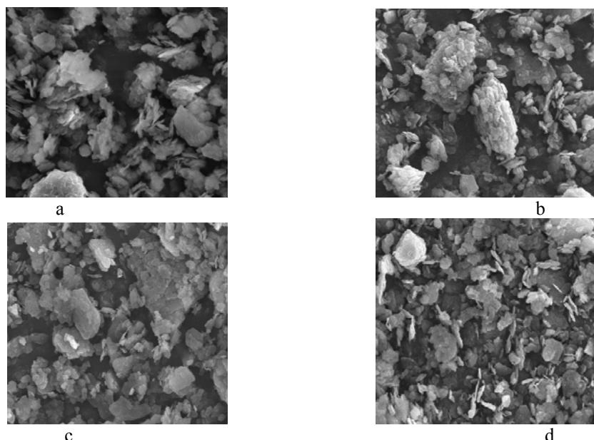
Fig. 1. SEM images of a) unmodified kaolin, b) kaolin modified with N-2-aminoethyl-3-aminopropyltriethoxysilane, c) kaolin modified with 3-metacryloxypropyltrimethoxysilane, d) kaolin modified with 3-aminopropyltriethoxysilane .
