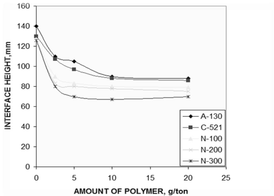
Fig. 2. Variation of interface height with the amount of polymer for  $20\mu\text{m}$  albite concentrate up on 5 in of settling time
