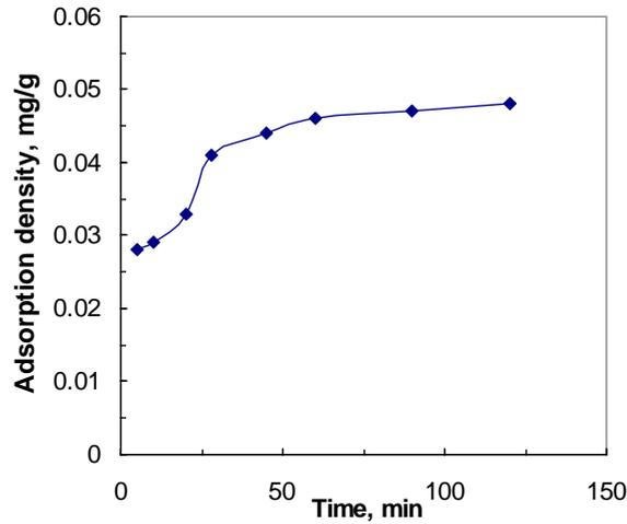
Fig. 10. Dependence of adsorption of 10 mg/kg N-300 on albite against conditioning time at natural pH
