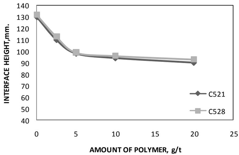
Fig. 4. Variation of interface height with the amount of cationic polymer for 20 µm albite concentrate up on 5 min of settling time
