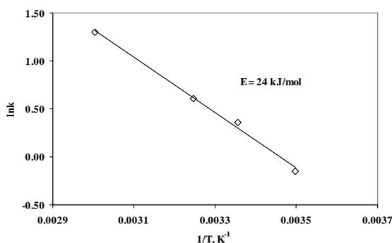
Fig. 8. Arrhenius plot for the dissolution of ulexite
