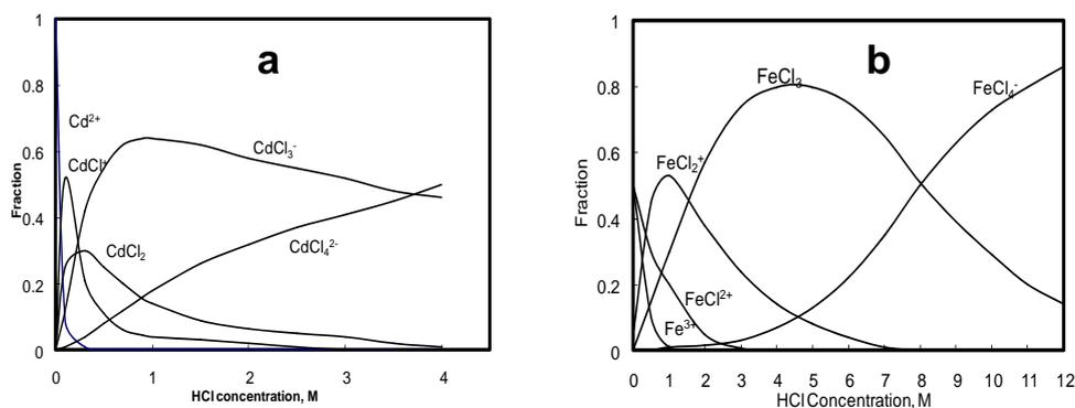
Fig. 1. Speciation diagram of Fe<sup>3+</sup> and Cd<sup>2+</sup> at different HCl concentrations
