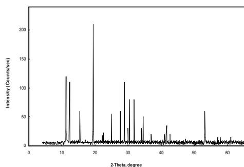
Fig. 4. X-ray diffraction analysis of the precipitated solids in phosphoric acid after addition of KCl
