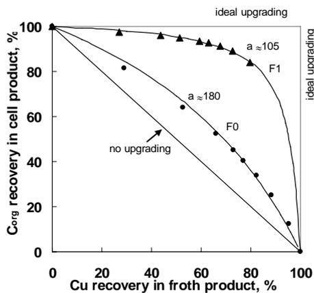
Fig. 7. Separation curve for laboratory batch tests on reflation of final industrial copper concentrates performed in the absence (F0) and presence (F1) of dextrin in the form of the Fuerstenaue upgrading curve
