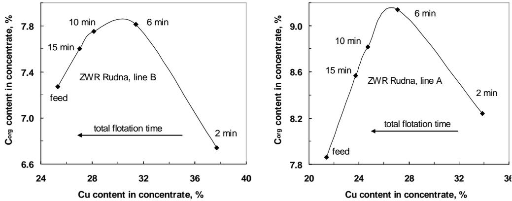
Fig. 2. Relation between organic carbon and copper content in the refloats in a laboratory flotation machine final industrial copper concentrate from side A and side B of ZWR Rudna (O/ZWR, 2009)
