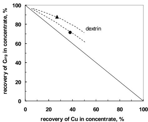
Fig. 4. The Fuerstenau upgrading curve showing relation between recovery of  $C_{org}$  in the cell product and Cu recovery in the froth product for industrial trial of reflation in the absence and presence of maltodextrin DE 6-8 at the dose of 1.93 kg/Mg. The throughput was 7640 Mg per shift, concentrate yield 6,84%
