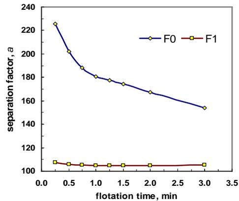
Fig. 6. Relation between separation factor  $a$ , reflecting separation of Cu and  $C_{org}$  during fractionated batch laboratory flotation, and flotation time. Results in the presence (F1) and in the absence (F0) of dextrin
