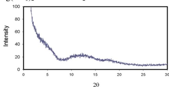
Fig.1. WAXS pattern of magnesium silicate – sample 5 (precipitated from 5%  $\text{MgSO}_4$  and 5%  $\text{SiO}_2$  sol)
