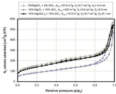
Fig. 4. N<sub>2</sub> adsorption/desorption isotherms of synthetic magnesium silicates (samples 5, 19 and 29)
