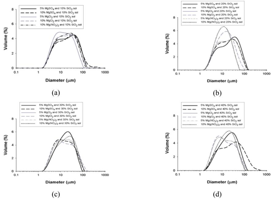
Fig. 2. PSD's of magnesium silicate – samples precipitated from (a) 10, (b) 20, (c) 30 and (d) 40% silica sol solution and different types and concentrations of magnesium salts
