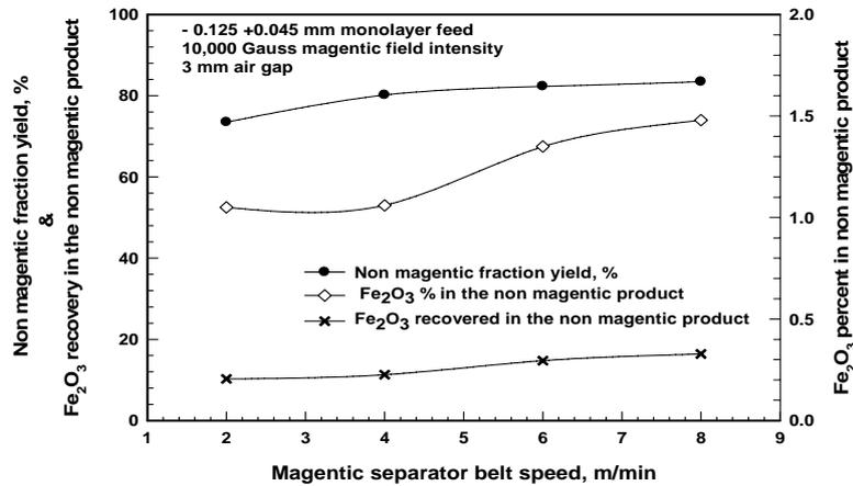
Fig. 4. Effect of main belt speed of "Dings" cross belt magnetic separator on the quantity and quality of nepheline syenite concentrate considering deslimed finer feed (-0.125+0.045 mm)
