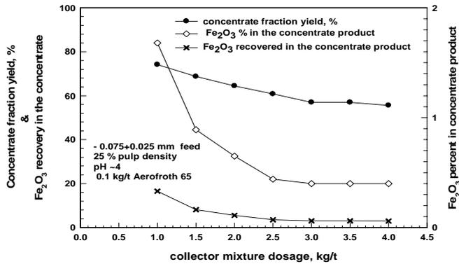
Fig. 5. Effect of dosage of Cynamid 801 and 825 as a collector on the quantity and quality of nepheline syenite concentrate
