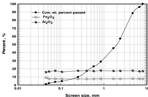
Fig. 1. Size distribution and chemical analyses of primary crushed nepheline syenite sample
