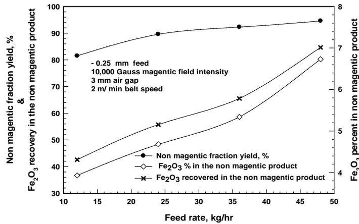
Fig. 3. Effect of the feed rate of "Dings" cross belt magnetic separator on the quantity and quality of nepheline syenite concentrate
