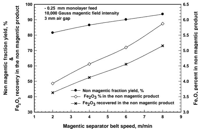
Fig. 2. Effect of the main belt speed of the "Dings" cross belt magnetic separator on the quantity and quality of nepheline syenite concentrate
