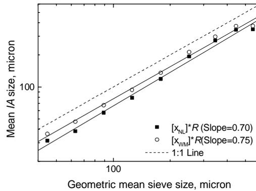
Fig. 6. IA means corrected by  $R$  against geometric mean of sieve fractions for number-based means (■) and volume (mass)-based means (○)
