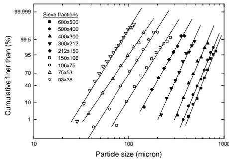
Fig. 1. Size distributions of sieve fractions plotted on log-normal drawing paper
