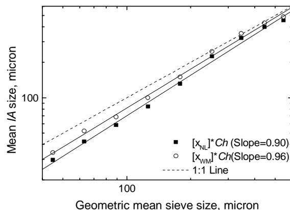
Fig. 5. IA means corrected by  $Ch$  against geometric mean of sieve fractions for number-based means (■) and volume(mass)-based means (○)
