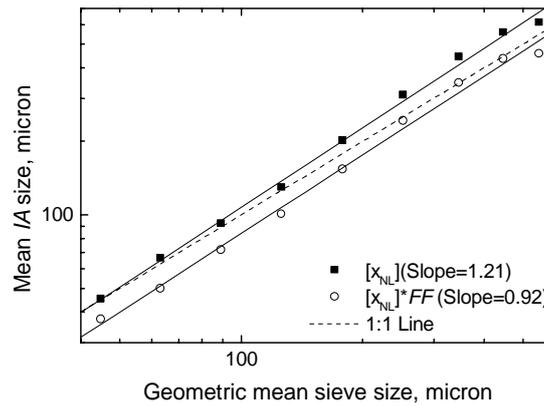
Fig. 3. Relationship between number-based IA means versus mean sieve sizes (■) and corrected number-based IA means by  $FF$  shape factor against geometric mean of sieve fractions (○)
