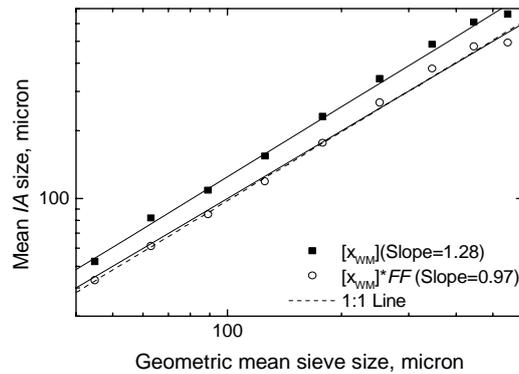
Fig. 4. Relationship between volume (mass)-based IA means versus mean sieve sizes (■) and corrected volume (mass)-based IA means by  $FF$  shape factor against geometric mean of sieve fractions (○)
