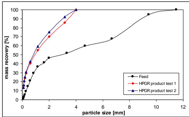
Fig. 3. Particle size distribution curves of feed and crushing products
