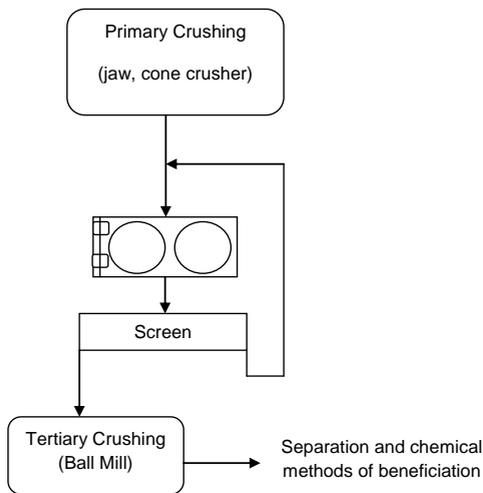
Fig. 1. Comminution circuit with HPGR device on second crushing stage (Saramak et al., 2010)
