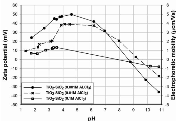
Fig. 4. Zeta potential versus pH of TiO<sub>2</sub>-SiO<sub>2</sub> for different ionic strength of AlCl<sub>3</sub>
