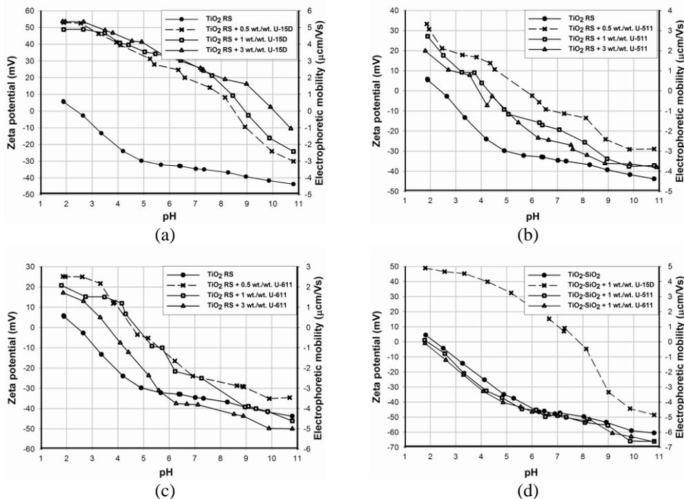
Fig. 2. Zeta potential and electrophoretic mobility versus pH for TiO<sub>2</sub> RS unmodified and modified with 0.5, 1 or 3 wt./wt. of (a) U-15D, (b) U-511, (c) U-611 and (d) for TiO<sub>2</sub>-SiO<sub>2</sub> oxide composite
