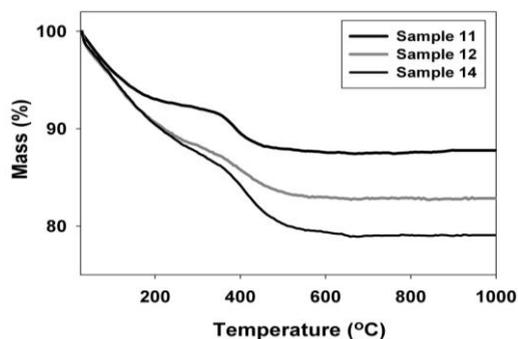
Fig. 10. TGA curves recorded for the unmodified silica precipitated in the emulsion system (Sample 11) and for the samples functionalised with octakis({3-glycidoxypropyl}dimethylsiloxy)octasilsesquioxanes (Samples 12 and 14)
