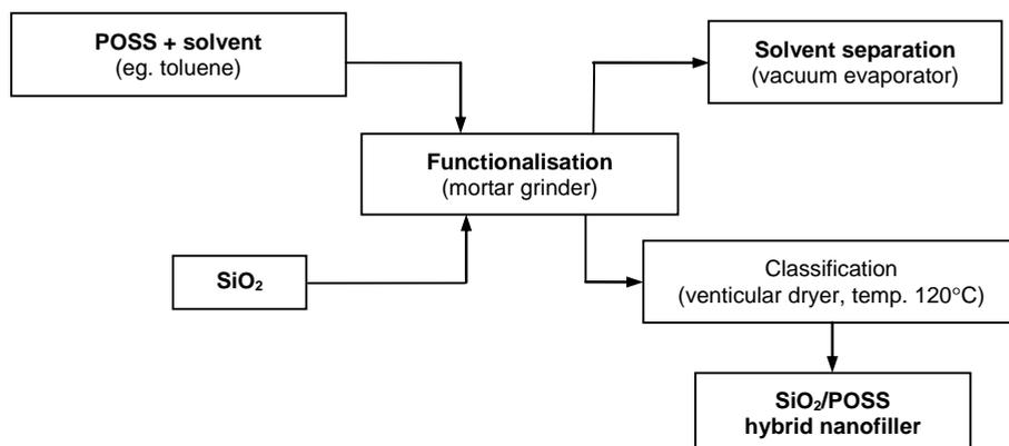
Fig. 3. Scheme of functional nanofillers mechanical preparation
