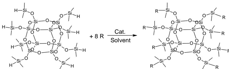
Fig. 2. Synthesis of octasubstituted polyhedral oligomeric silsesquioxanes
