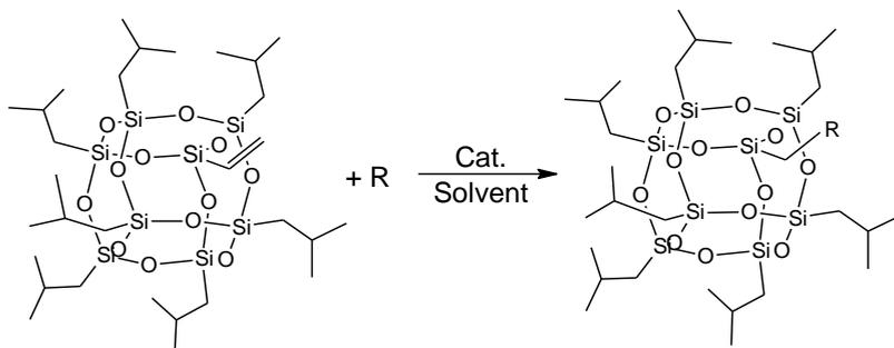
Fig. 1. Synthesis of monosubstituted polyhedral oligomeric silsesquioxanes
