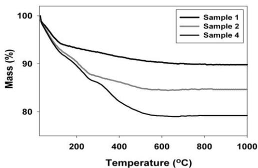
Fig. 9. TGA curves for the unmodified hydrated silica (Sample 1) and hybrids functionalised with octakis({3-glycidoxypropyl}dimethylsiloxy)octasilsesquioxanes (Samples 2 and 4)
