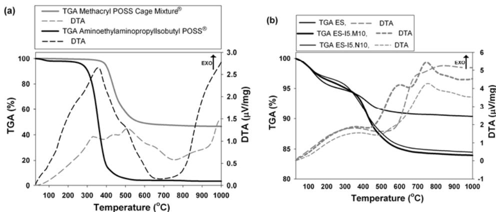
Fig. 5. Thermograms of (a) pure Methacryl POSS<sup>®</sup> Cage Mixture and Aminoethylaminopropylisobutyl POSS<sup>®</sup> and (b) unmodified emulsion silica, and hybrids functionalization with 5 weight parts by mass of isocyanatosilane and 10 weight parts by mass of selected POSS compounds
