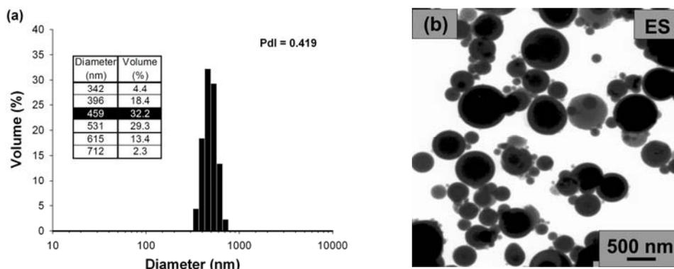
Fig. 6. PSD (a) and TEM microphotograph (b) of the unmodified SiO<sub>2</sub> precipitated in the emulsion system
