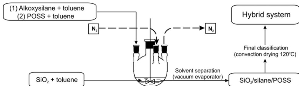
Fig. 1. Schematic diagram of  $\text{SiO}_2/\text{silane}/\text{POSS}$  hybrid systems preparation
