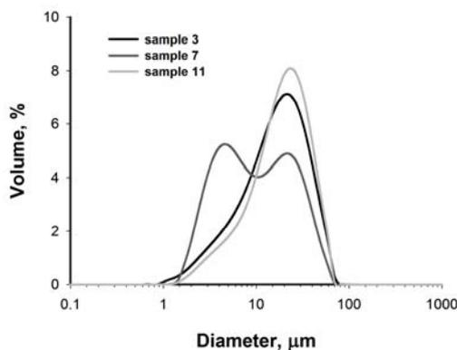
Fig. 3. Particle size distributions (Mastersizer 2000) of selected biocomposites
