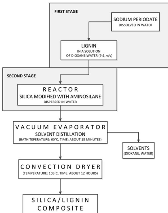
Fig. 1. Preparation of silica/lignin biocomposites – a schematic representation
