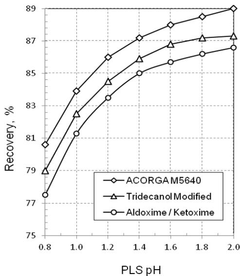
Fig. 6. SX circuit recovery comparison (30 vol % extractant, 25 g/dm<sup>3</sup> of copper in PLS) (Moore et al., 1999)
