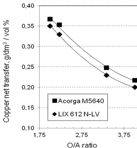
Fig. 4. Copper net transfer in organic at 30 vol % of reagent as a function of overall extraction O/A ratio, PLS II
