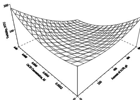
Fig. 8. Effect of A-150 amount and  $\text{CaCl}_2 \cdot 2\text{H}_2\text{O}$  concentration on turbidity (pH 7)
