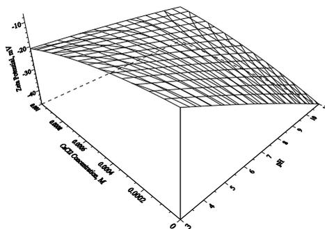
Fig. 6. Effect of pH and  $CaCl_2 \cdot 2H_2O$  concentration on zeta potential (A-150: 400 g/Mg)
