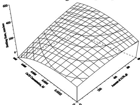
Fig. 7. Effect of A-150 amount and  $\text{CaCl}_2 \cdot 2\text{H}_2\text{O}$  concentration on settling rate (pH 7)
