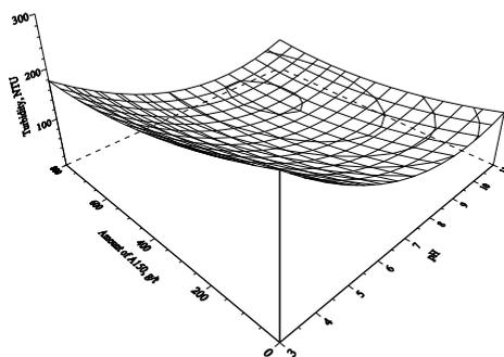
Fig. 2. Effect of pH and A-150 amount on turbidity ( $\text{CaCl}_2 \cdot 2\text{H}_2\text{O}$ : 0.0005 M)
