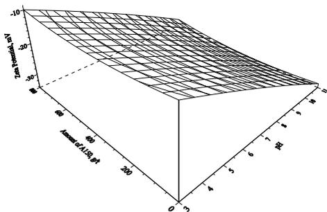
Fig. 3. Effect of pH and A-150 amount on zeta potential ( $\text{CaCl}_2 \cdot 2\text{H}_2\text{O}$ : 0.0005 M)
