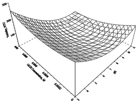
Fig. 5. Effect of pH and  $CaCl_2 \cdot 2H_2O$  concentration on turbidity (A-150: 400 g/Mg)
