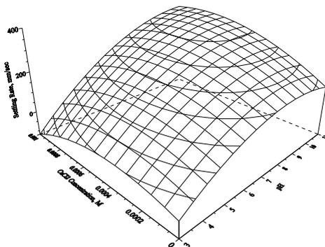
Fig. 4. Effect of pH and  $\text{CaCl}_2 \cdot 2\text{H}_2\text{O}$  concentration on settling rate (A-150: 400  $\text{g} \cdot \text{t}^{-1}$ )
