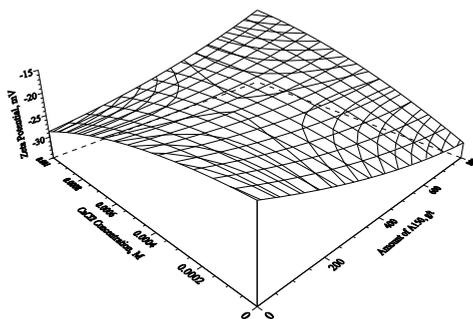
Fig. 9. Effect of A-150 amount and  $\text{CaCl}_2 \cdot 2\text{H}_2\text{O}$  concentration on zeta potential (pH 7)
