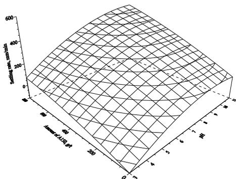
Fig. 1. Effect of pH and A-150 amount on settling rate ( $\text{CaCl}_2 \cdot 2\text{H}_2\text{O}$ : 0.0005 M)
