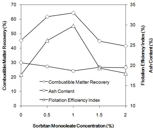
Fig. 4. Flotation results of lignite pre-treated by sorbitan monooleate
