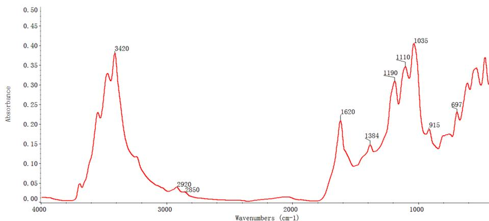
Fig. 1. FTIR spectrum of lignite
