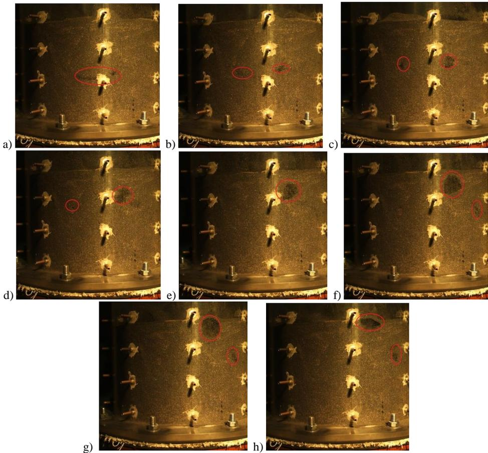
Fig. 4. Bubble behavior caused by plugged holes in air distributors
