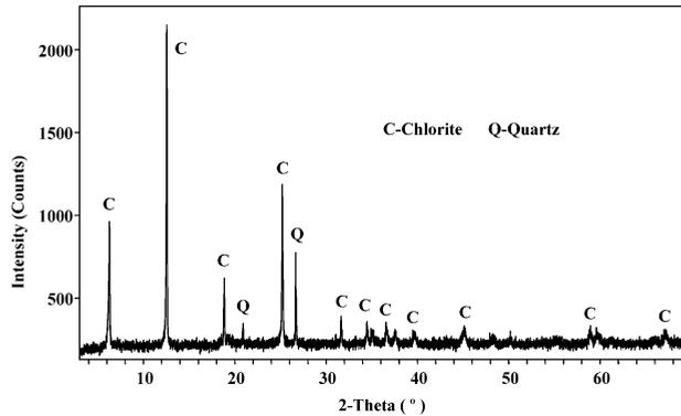
Fig. 1. X-ray diffraction pattern of the chlorite sample
