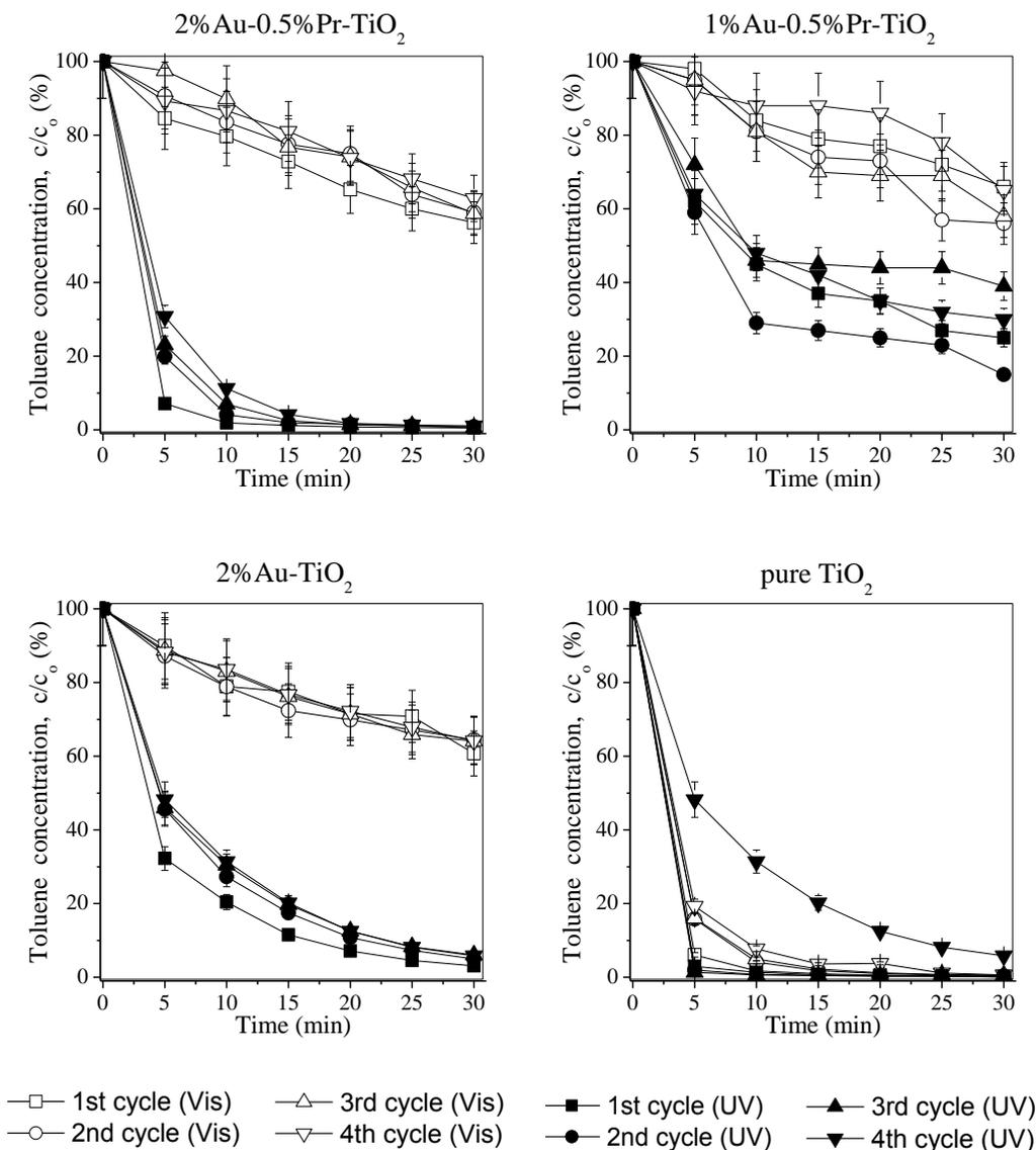
Fig. 4. Efficiency of toluene removal from gas phase in four subsequent cycles in the presence of Au-Pr-TiO<sub>2</sub>, Au-TiO<sub>2</sub> and pure TiO<sub>2</sub> under UV or Vis irradiation
