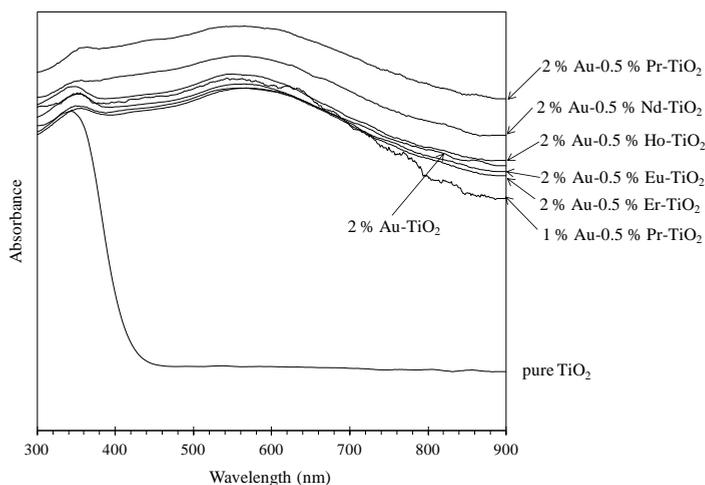
Fig. 2. Diffuse reflectance spectroscopy spectra of Au-RE-TiO<sub>2</sub> photocatalysts
