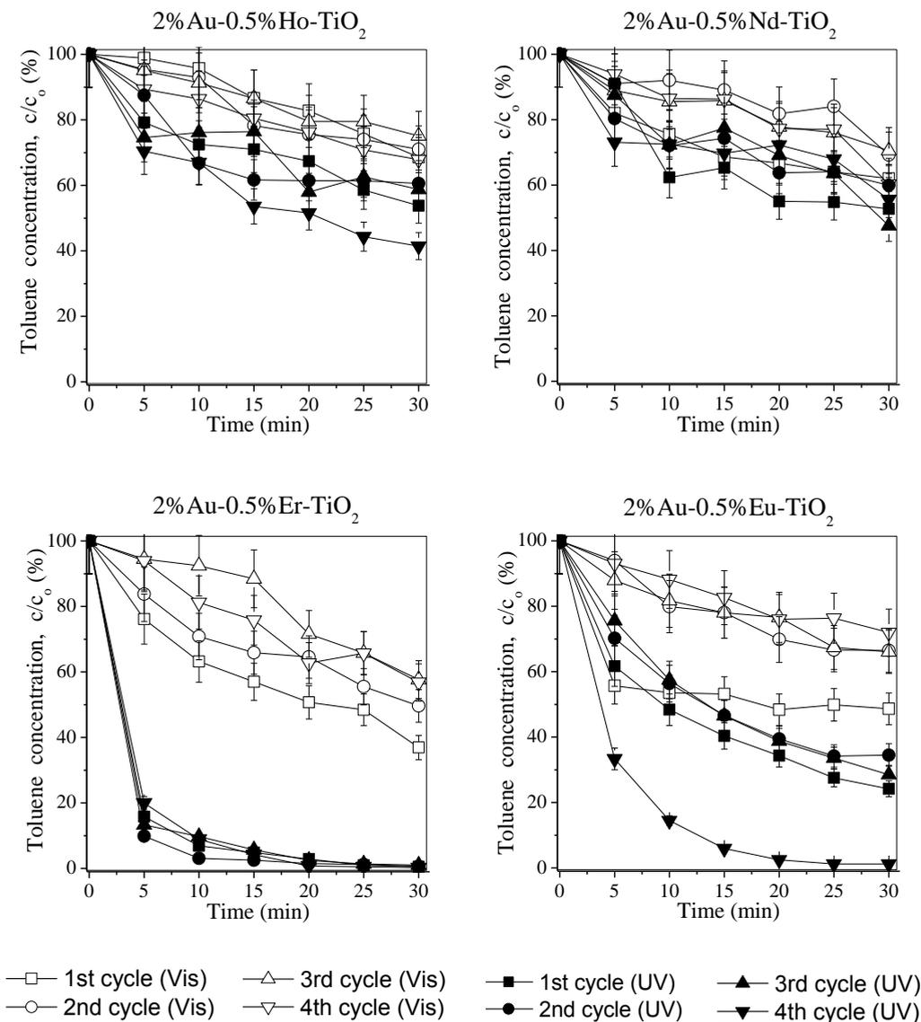
Fig. 3. Efficiency of toluene removal from gas phase in four subsequent cycles in the presence of Au-RE-TiO<sub>2</sub> under UV or Vis irradiation
