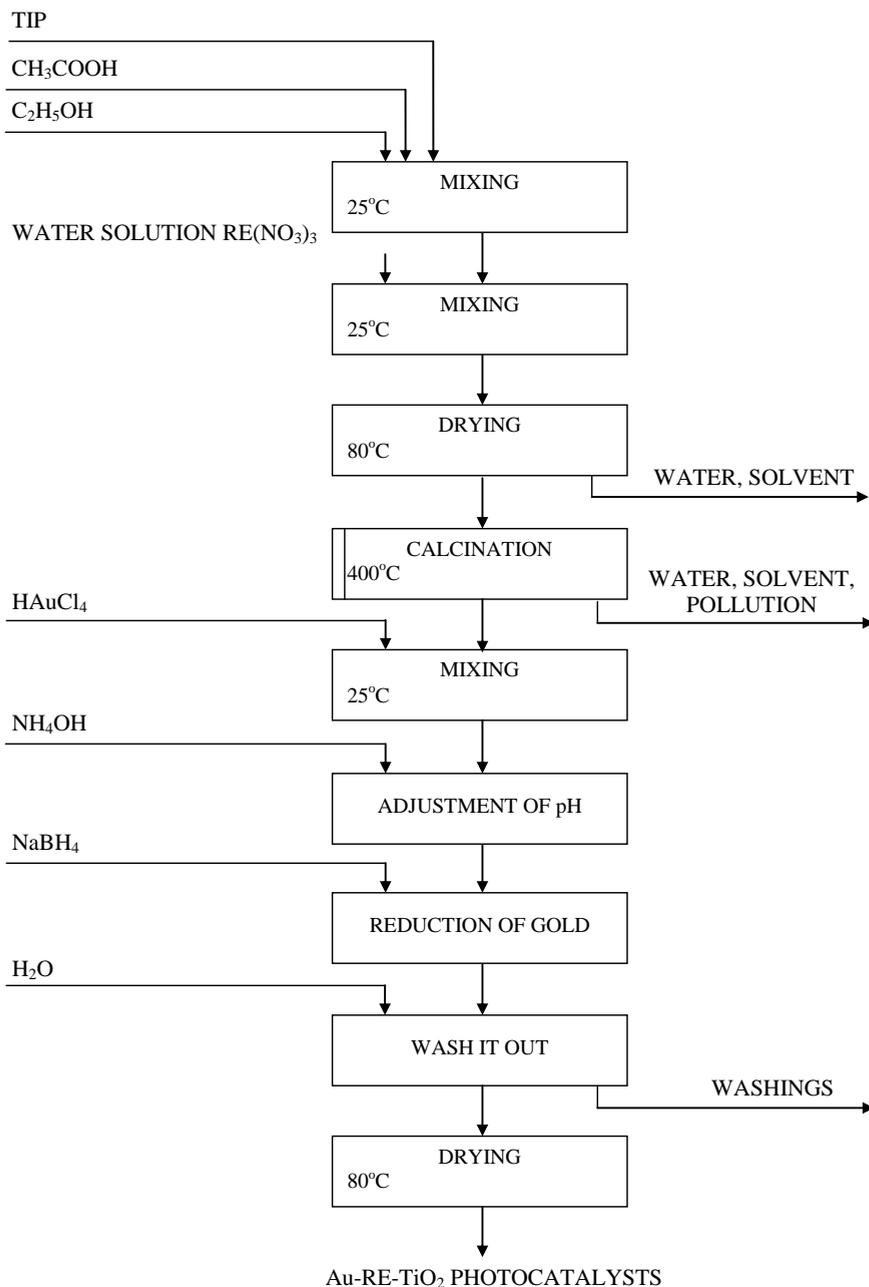
Fig. 1. Block diagram of preparation of Au-RE-TiO<sub>2</sub> photocatalysts
