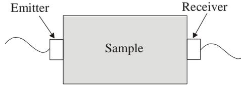
Fig. 1. The method of measuring P-wave velocity
