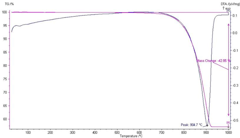
Fig. 6. The TG-DTA curve for  $L_y$  decomposition
