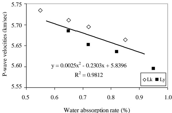
Fig. 3. Correlation of P-wave velocity vs. water absorption rate
