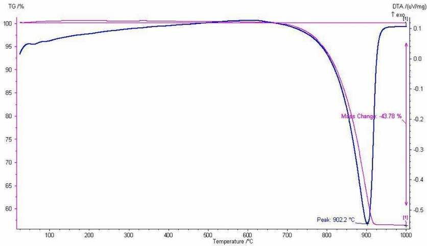
Fig. 5. The TG-DTA curve for  $L_k$  decomposition
