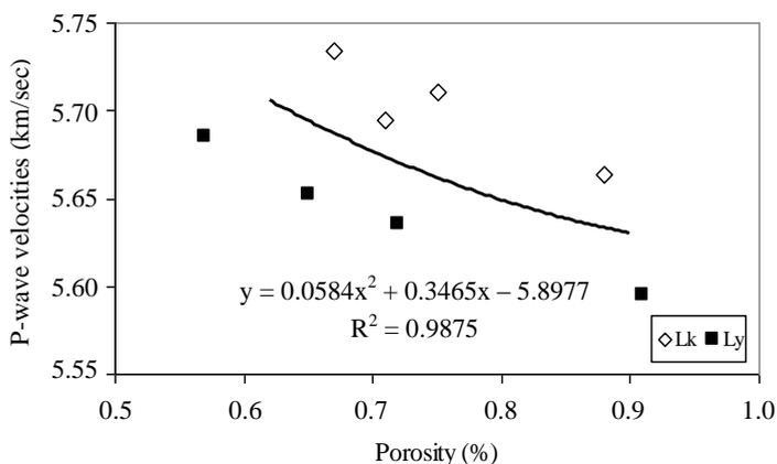
Fig. 4. Correlation of P-wave velocity vs. porosity
