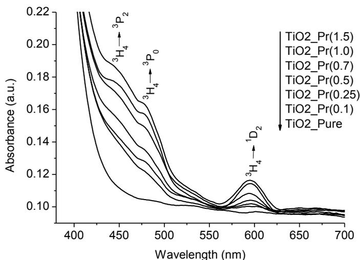
Fig. 2. Absorption properties of Pr-TiO<sub>2</sub> prepared by the sol-gel method
