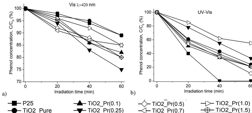
Fig. 4. Efficiency of phenol photodegradation in the presence of Pr-doped TiO<sub>2</sub> during irradiation light: a) Vis ( $\lambda > 420$  nm), b) UV/Vis
