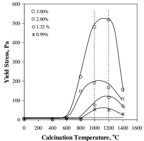
Fig. 6. Yield stress of bentonite suspensions with calcinated MgCO<sub>3</sub> depending on the MgO addition (at legend) and calcination temperature at shear rate of 93 s<sup>-1</sup>
