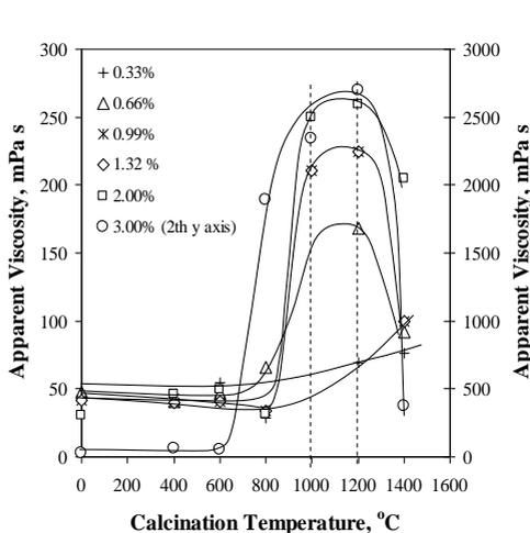
Fig. 5. Apparent viscosities of bentonite suspensions (solid ratio is 4.75 %) with calcinated MgO<sub>3</sub> depending on the MgO addition (at legend) and calcination temperature at shear rate of 93 s<sup>-1</sup>
