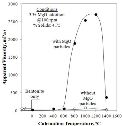
Fig. 10. Apparent viscosities of bentonite suspensions in the presence of  $MgCO_3$  calcinated at various temperatures
