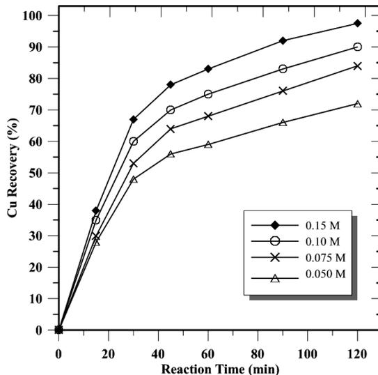
Fig. 1. Effect of the nitrite concentration on copper recovery. Initial electrolyte conditions:  $\text{C}_{\text{H}_2\text{SO}_4} = 1 \text{ M}$ ,  $d_{\text{mean}} = 15 \mu\text{m}$ ,  $T = 120^\circ\text{C}$ ,  $P_{\text{tot}} = 6 \text{ atm}$
