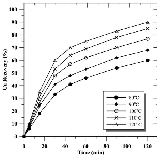
Fig. 2. Effect of the temperature on copper recovery. Initial electrolyte conditions:
