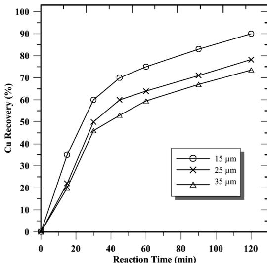
Fig. 3. Effect of the particle size of concentrate on copper recovery. Initial electrolyte conditions:
