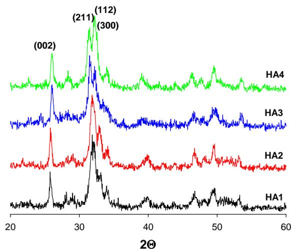
Fig. 3. XRD diffraction patterns of hydroxyapatite structures
