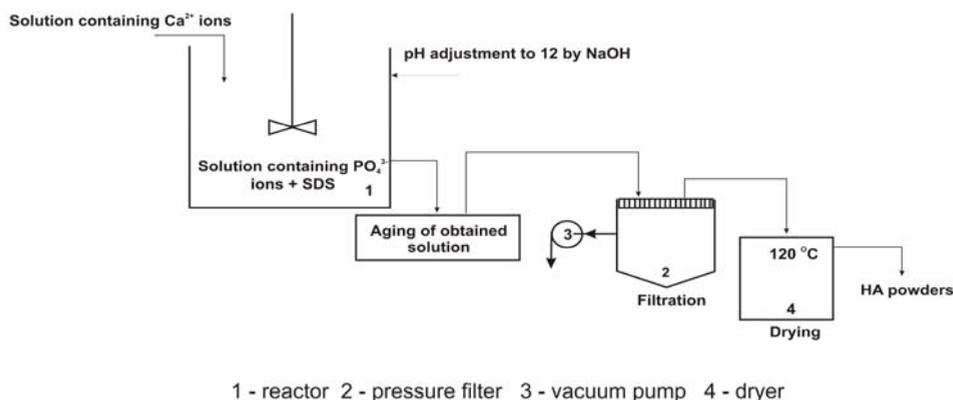
Fig. 1. Preparation of hydroxyapatite – a schematic presentation
