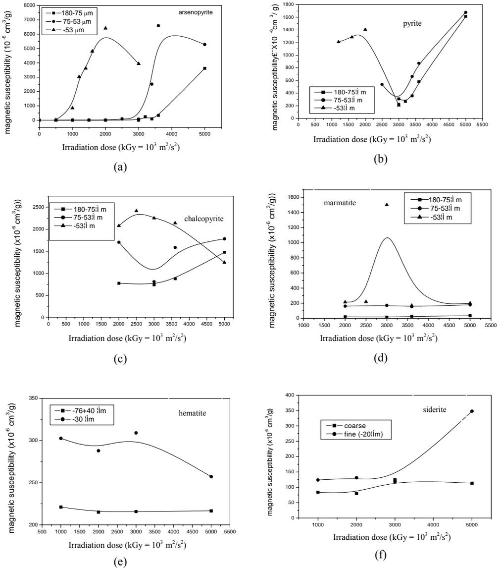
Fig. 1. Magnetic susceptibility of arsenopyrite (a), pyrite (b), chalcopyrite (c), marmatite (d), hematite (e) and siderite (f) as a function of irradiation dose
