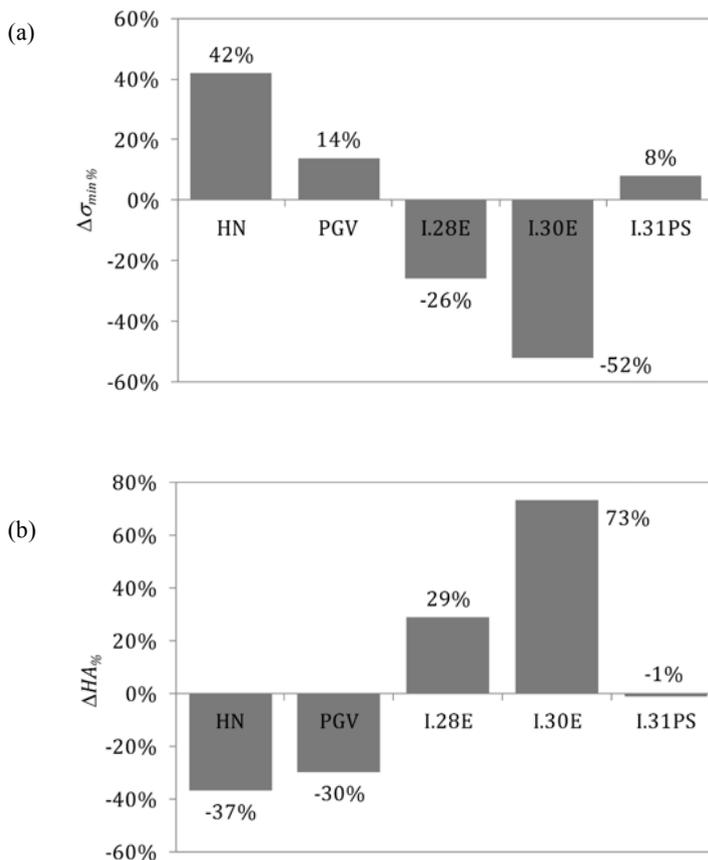
Fig. 4. Relative change of (a) – the minimum surface tension ( $\Delta\sigma_{min}\%$ ) and (b) – the hysteresis area ( $\Delta HA\%$ ) for different mineral nanoparticles at concentration of  $0.5 \text{ mg/cm}^3$
