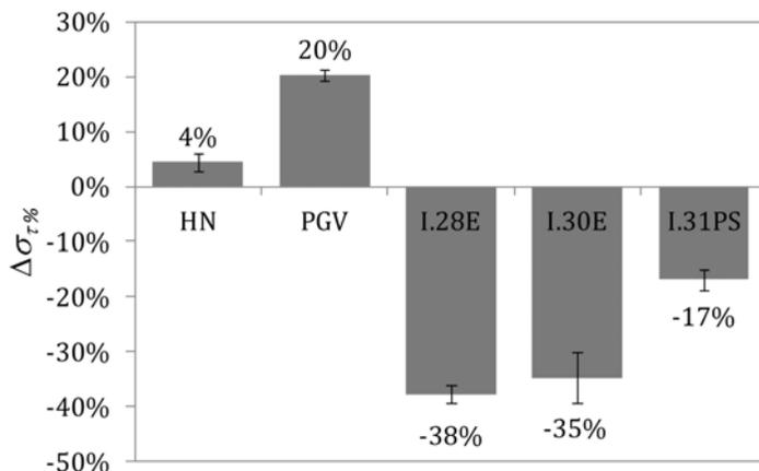
Fig. 7. Comparison of  $\Delta\sigma_{\tau\%}$  value for PS with different mineral nanoparticles (0.5 mg/cm<sup>3</sup>).
