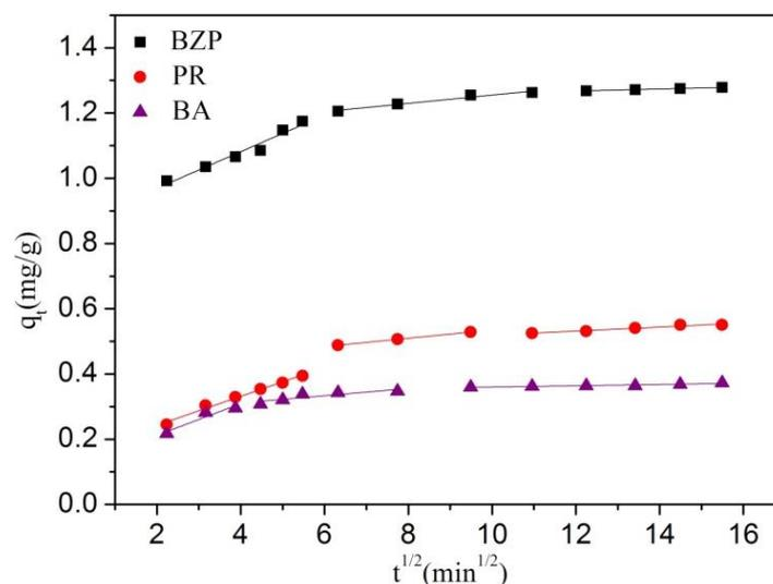
Fig. 2. Intra-particle diffusion model of PR, BZP and BA adsorption by PC
