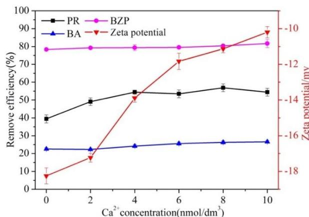
Fig. 5. Zeta potential of PC in different  $\text{Ca}^{2+}$  concentration and its influence on pollutants removal (Initial concentration  $30 \text{ mg/dm}^3$ ; adsorbent dosage  $20 \text{ g/dm}^3$ ; natural pH 7.1; temperature 293 K)
