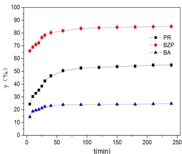
Fig. 1. Adsorption kinetics of PR, BZP and BA on PC (initial concentration 30 mg/dm<sup>3</sup>; adsorbent dosage 20 g/dm<sup>3</sup>; natural pH 7.1; temperature 20 °C)
