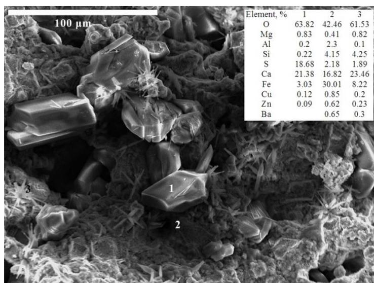
Fig. 2. SEM-EDS analysis of Ca100 sample of the Waelz slag
