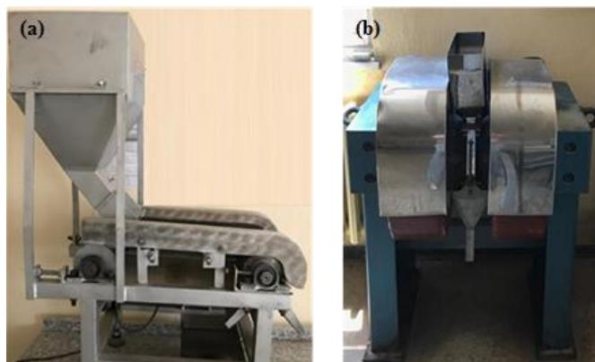
Fig. 3. Laboratory scale (a) dry high gradient belt magnetic separator (b) wet high gradient magnetic separator
