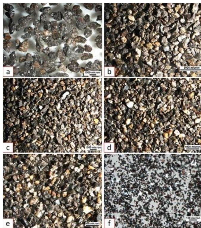
Fig. 2. Pictures of different size fractions (a) 2-1 mm (b) 1000-600  $\mu\text{m}$  (c) 600-400  $\mu\text{m}$
