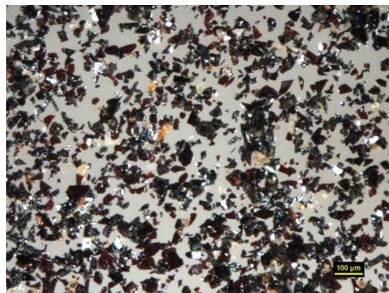
Fig. 6. Picture of the  $-45\text{ }\mu\text{m}$  fraction of concentrate produced from single stage beneficiation process by HGMS
