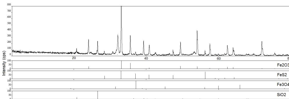
Fig. 1. XRD diffractogram of micaceous iron oxide ore
