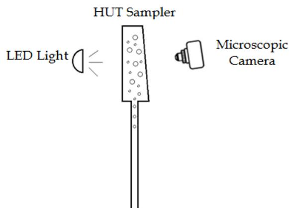
Fig. 1. Image acquisition apparatus for bubble size distribution analysis
