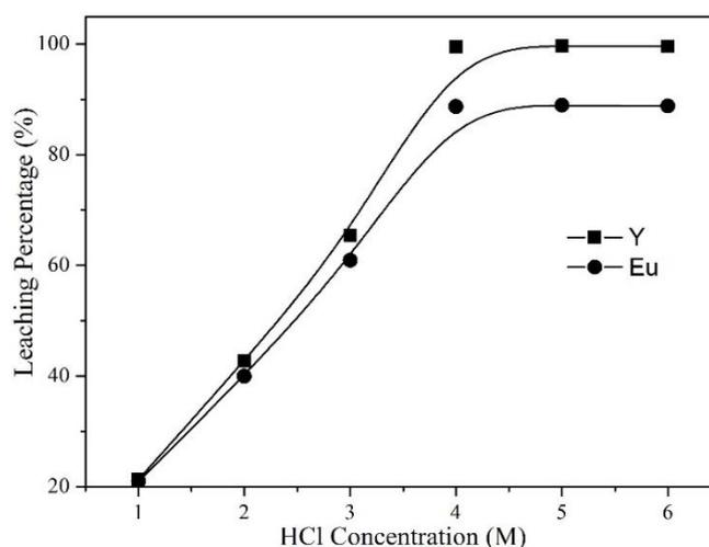
Fig. 3. Effect of HCl concentration on leaching percentage of Y and Eu ( $\text{H}_2\text{O}_2$ :  $0.2 \text{ cm}^3/\text{g}$  T:  $60 \text{ }^\circ\text{C}$ , t: 180 min, L/S:  $10 \text{ cm}^3/\text{g}$ )
