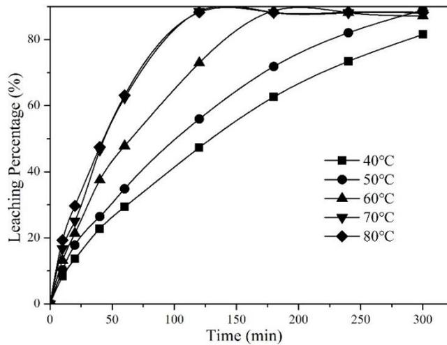
Fig. 9. Effect of temperature on leaching percentage of Eu at different reaction times (acid: 4 M HCl, H<sub>2</sub>O<sub>2</sub>: 0.2 cm<sup>3</sup>/g, L/S: 7.5 cm<sup>3</sup>/g)
