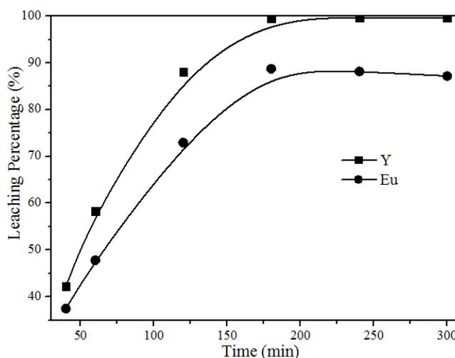
Fig. 6. Effect of reaction time on leaching percentage of Y and Eu (acid: 4 M HCl, H<sub>2</sub>O<sub>2</sub>: 0.2 cm<sup>3</sup>/g, T: 60 °C, L/S: 10 cm<sup>3</sup>/g)
