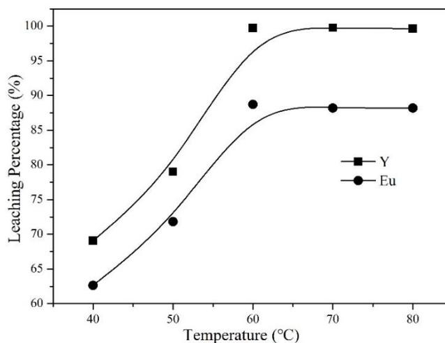
Fig. 5. Effect of temperature on leaching percentage of Y and Eu (acid: 4 M HCl, H<sub>2</sub>O<sub>2</sub>: 0.2 cm<sup>3</sup>/g, t: 180 min, L/S: 10 cm<sup>3</sup>/g)
