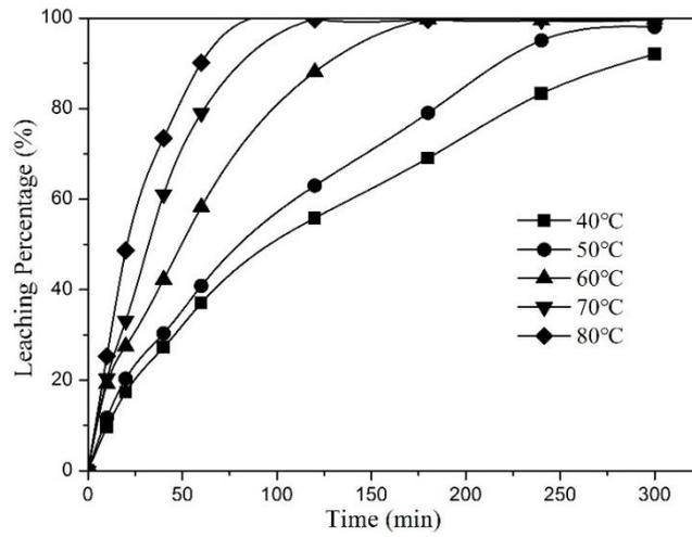
Fig. 8. Effect of temperature on leaching percentage of Y at different reaction times (acid: 4 M HCl, H<sub>2</sub>O<sub>2</sub>: 0.2 cm<sup>3</sup>/g, L/S: 7.5 cm<sup>3</sup>/g)
