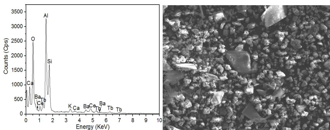
Fig. 14. SEM-EDS analysis of leaching residue at 180 min
