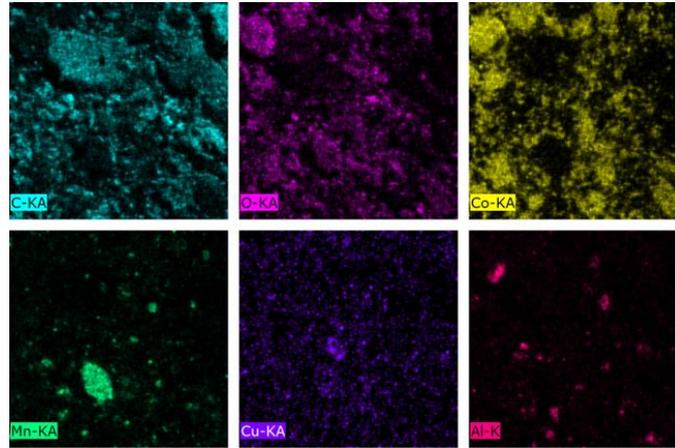
Fig. 2. Surface element distribution of Fig. 1(a)
