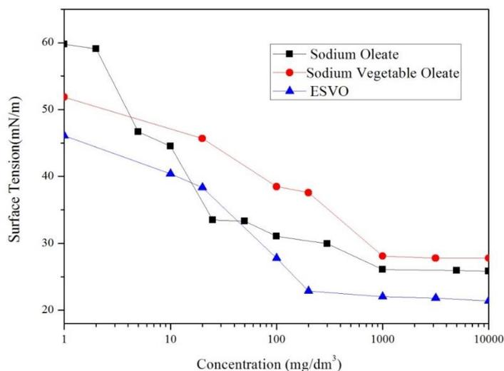
Fig. 5. Surface tension of collectors with different concentration
