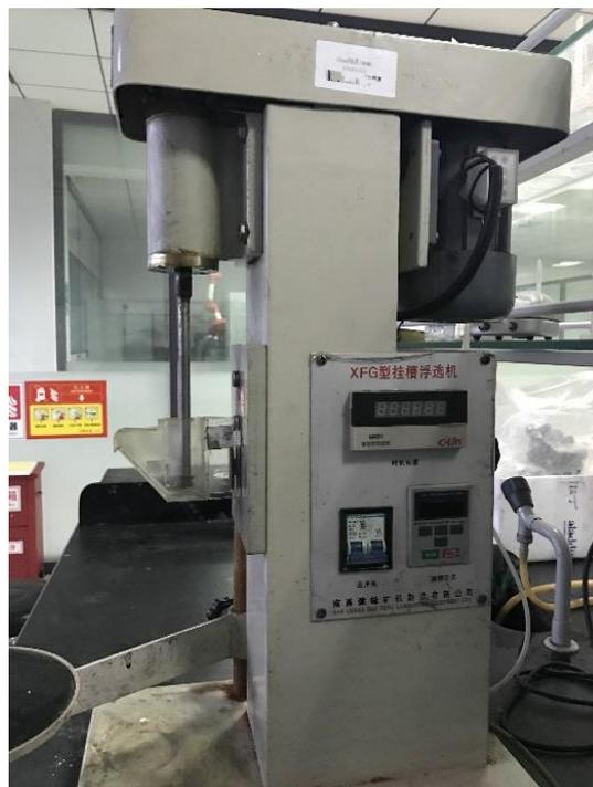
Fig. 1. XFG micro-flotation machine
