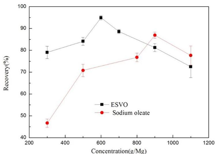
Fig. 4. Relationship between the recovery of fluorite and the collector concentration ( $\text{pH}_{\text{ESVO}} = 6$ ,  $\text{pH}_{\text{sodium oleate}} = 8$ )
