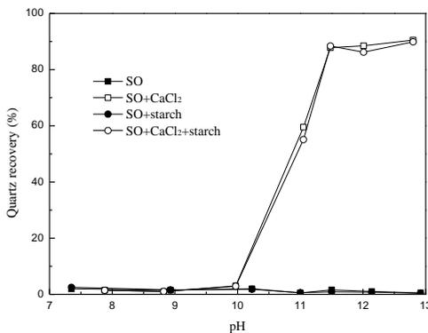
Fig. 2. Quartz recovery in froth product as a function of pH (sodium oleate (SO) 160 mg/dm<sup>3</sup>, calcium chloride 100 mg/dm<sup>3</sup>, starch 60 mg/dm<sup>3</sup>)
