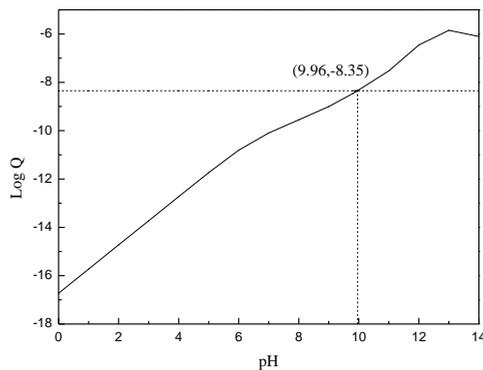
Fig. 9. Log Q as a function of pH in CaCl<sub>2</sub>-NaOH-siderite system (C<sub>(CaCl<sub>2</sub>)</sub> = 100 mg/dm<sup>3</sup>, log K<sub>sp,CaCO<sub>3</sub></sub> = -8.35)
