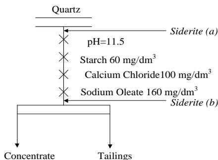
Fig. 1. Flowsheet and corresponding flotation conditions of test
