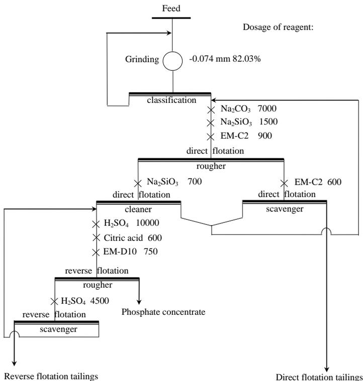
Fig. 3. Flow chart of scale-up flotation test
