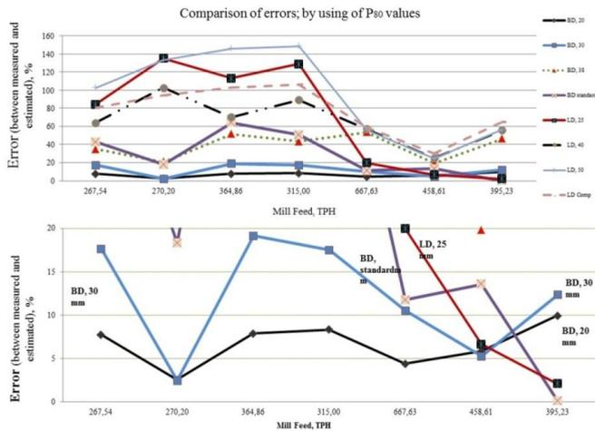
Fig. 5. Comparison of errors using  $P_{80}$  values
