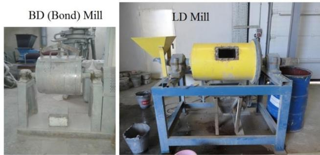
Fig. 3. BD and LD laboratory ball mills
